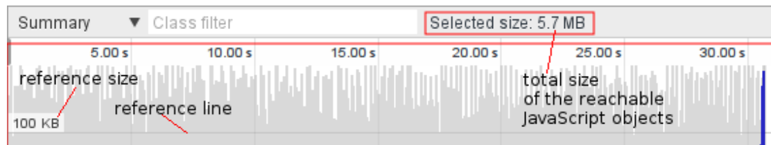
Figure 5.13: Example heap allocation record; note that this was recorded over about 30 seconds
