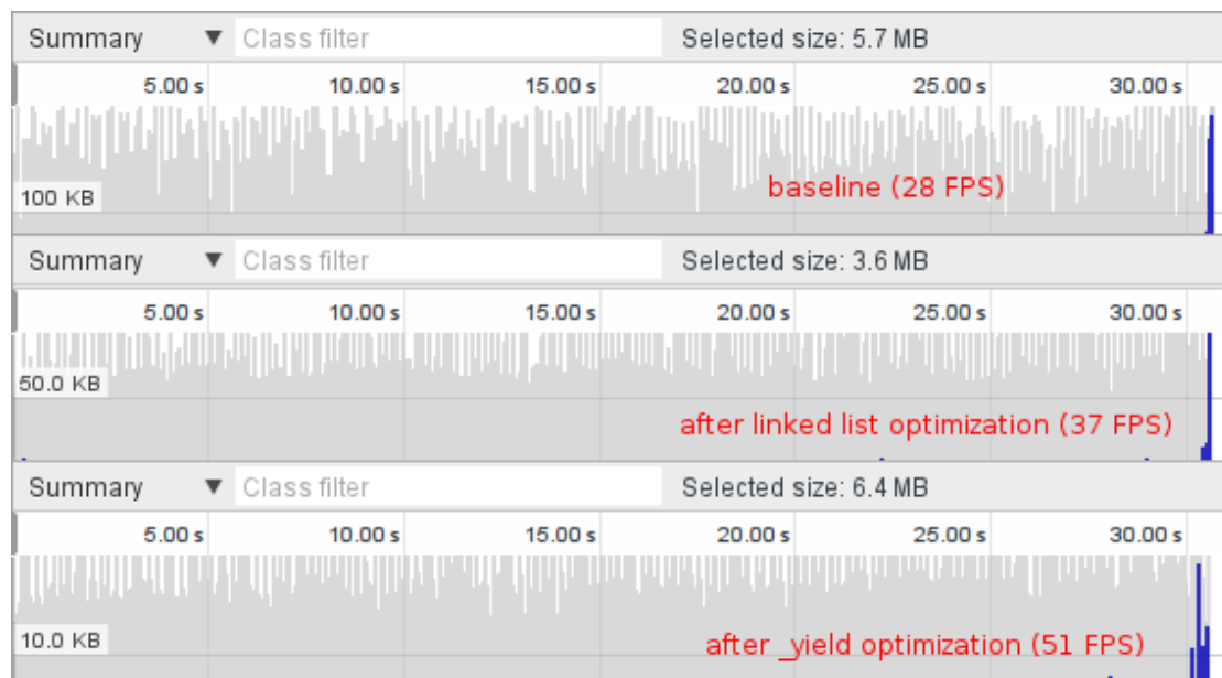
Figure 5.44: The optimizations decreased the amount of memory used by the benchmark (note the reference size: 100, 50, and 10 KB)
